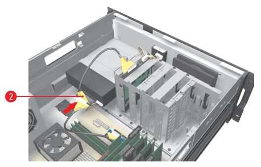
Figure 14. Installing DVD-RW Data Cable
